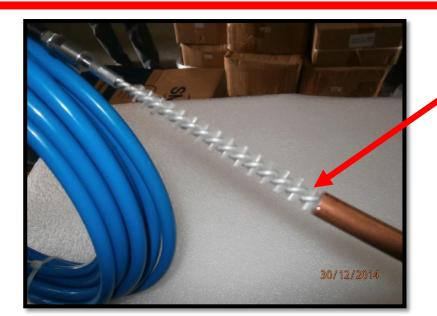
If the brush is too tight for insertion, trimming of the brush is needed!
