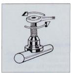
After extraction, set the correct insert depth for the tube dia. with the cam pincer
