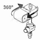
5. Press firmly to ensure coil is secured.
