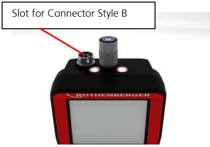
Figure 5 – Cable Connections (Connector Style B, Silver Color)
