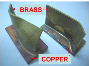
: Blockade FC 2mm Dia. (Flux-Coated) (AWS BCuP-9)
