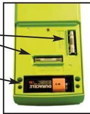
**Separate Battery Compartment**
