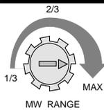
It is necessary to carry out a thorough walk test of the detector to ensure that the correct coverage is being achieved and no over spill of the microwave is occurring. Also to ensure that both PIR & microwave are working to the same detection area.
