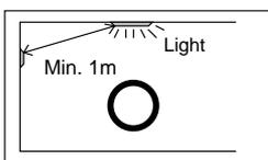
Locate the detector at least 1 meter away from any illumination to avoid possible interference to microwave sensor.
