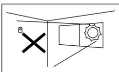
Do not install where the detector is in or facing direct/reflected sunlight, windows onto main roads (car head lights) or strong draughts / heaters.
