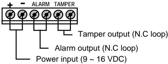
☞ *TAMPER terminals should be connected to the 24-hour N.C supervisory loop of control panel.*
