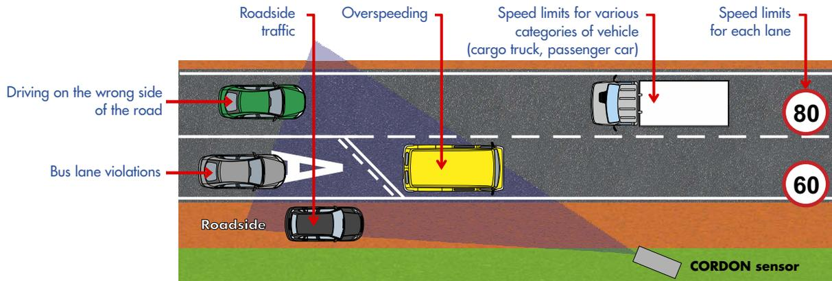
The violation data includes the recognized license plate number, measured speed, type of violation (speeding, roadside driving, bus lane driving or driving in wrong direction), movement direction, date and time of violation, speed limit for current road section, name of controlled road section, geographical coordinates, sensor serial number.
