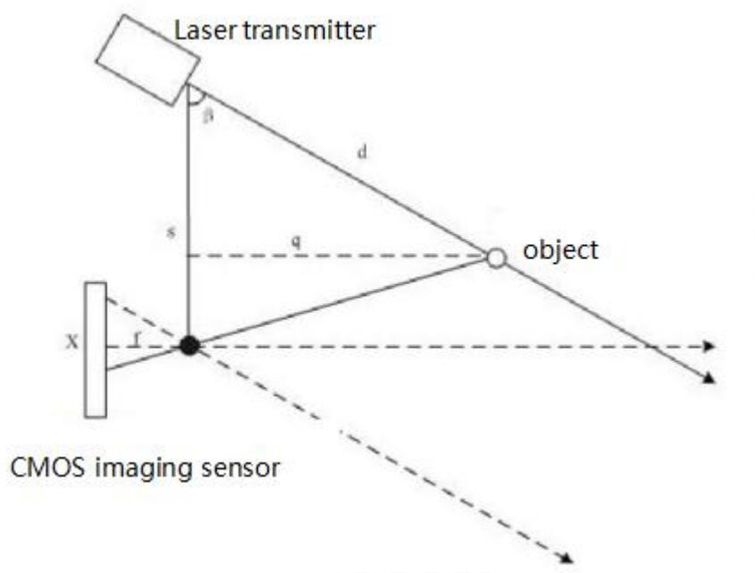
Through the instant calculation of the embedded signal processing module in LS01B, data of distance between the object and LS LIDAR, together with relative direction angle, will be output from the communication interface.
