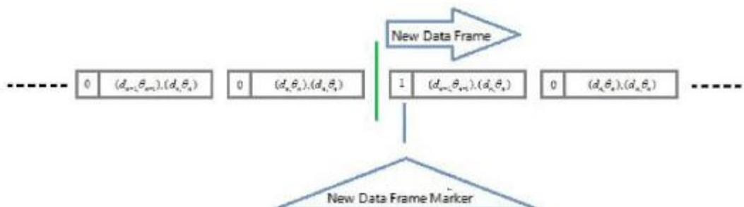
The detecting data of LS01B are output in message format showed above, instructions from external system can start and stop the data output of LS01E or configure the format of output data.
