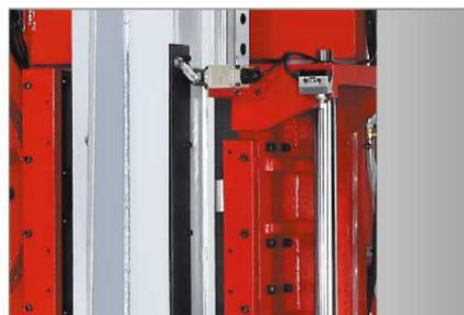
**Linear Guides used for Saw Bow and Table Movement**
