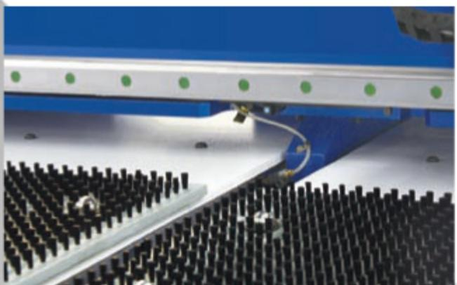
Provides overall protection to the clamps. Protects the clamps from striking or being punched when manually moved to this critical area or in case of a software protection failure.
