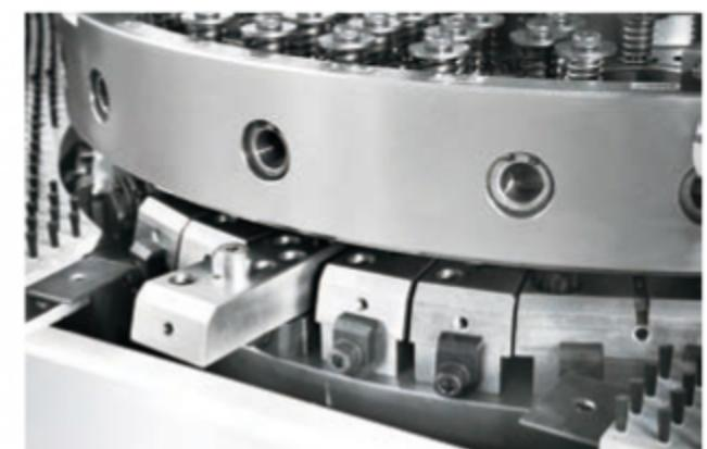
**Material feeding structure and clamps****Matériel de chargement et serres**
