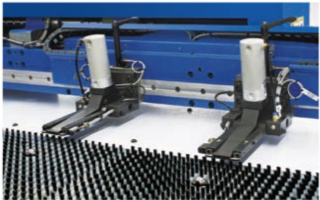
Long stroke precision ground ball screw, four guiding-slots linear guide, higher positioning precision, faster speed.
