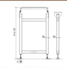
Material: 50 x 50mm x 2.3t Mild Steel SHS Height (H): 400 ~ 2000mm +/- 25mm (in 50mm increments)
