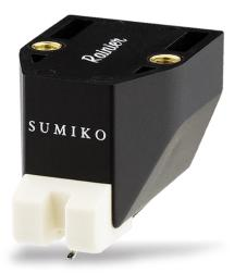
The Rainier has a simple elliptical stylus (only in relation to the higher cartridges in the series; no elliptical stylus is truly simple), and its cantilever is an aluminum pipe. Its specifications include a frequency response of 15Hz-25kHz, channel separation of 25dB at 1kHz, channel balance of 1.5dB at 1kHz, and output of 5.0mV. The range of vertical tracking force (VTF) is 1.8-2.2gm, with 2.0gm as the recommended value.
