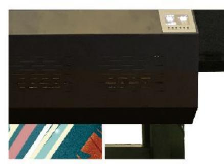
Infrered heater and cooling fan. Make sure the picture dries quickly.
