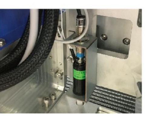
Dual mute THK guide rails ensure stability of printing and high quality printing output. The sheet media is automatically positioned, and the assistance of the front pressure bar makes the material more smooth, ensuring the accuracy of printing. Automatic height measurement system, adjust the distance between the baseplate and the media automatically to guarantee the best quality.
