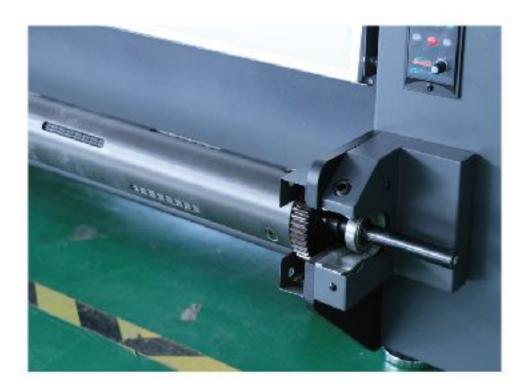
Integrated belt & flatbed media feeding system is competent to print both roll and rigid media. Folding extension frame saves space and cost as well. Independent widened platform Is able to accommodate more materials. Air-shaft take up system makes more stable paper collecting.
