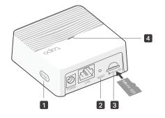
**1** SYNC Button Press to pair with the camera, or silence the hub when it rings.
