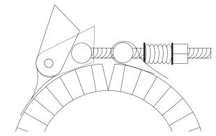
**Latch And Trunion Clamps** provide a quick clamp option. Clamping force is similar to barrel clamps and a spring is included to allow for thermal expansion of metals.
