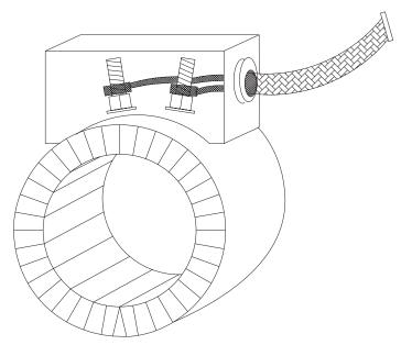
**SS Braid** method includes a loose metal braid that is welded to the terminal box with a coupler. This provides excellent abrasion protection and flexibility. Leads are attached to posts with a ring connectors.
