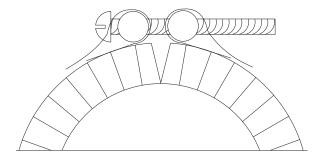
**Barrel Clamps** are used in applications where access for instrumentation is required. Includes an oversized gap.
