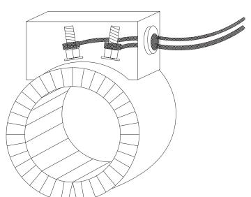
**Flexible Lead Wire** exits tangential to heater and includes leads connected to the post terminals with ring connectors. This termination method requires a terminal box.
