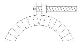
**Clamp Tabs** are a standard clamping option that offer a uniform clamping force across the heater width.
