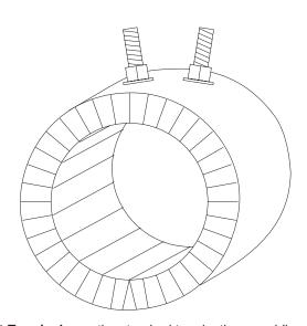
Post Terminals are the standard termination, providing quick connection with ring or fork connectors or buss strips, ¼ - 20 inch thread, and includes double nuts and washers. Standard terminal location is 180° from gap.
