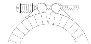
**Spring Loaded Barrel Clamps** help to compensate for the thermal expansion of metals.
