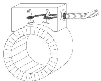
Flexible SS Hose is welded to the terminal box with a coupler.
