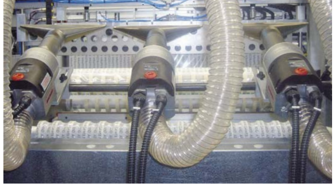
Three LHS 60S air heaters with wide slot nozzles in a wrapping line.
