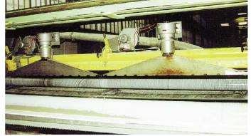
Two air heaters and two blowers used to dry impregnated Eternit piping. Two wide slot nozzles ensure the air is evenly distributed.
