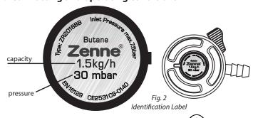
The "Snap On Compact" is a domestic regulator designed to supply gas to appliances. The pressure and capacity are indicated on the identification label (Fig.2).
