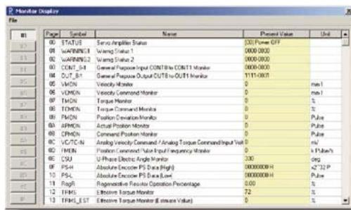
a. Monitor Display : Observe Operation and Input/Output signal status
