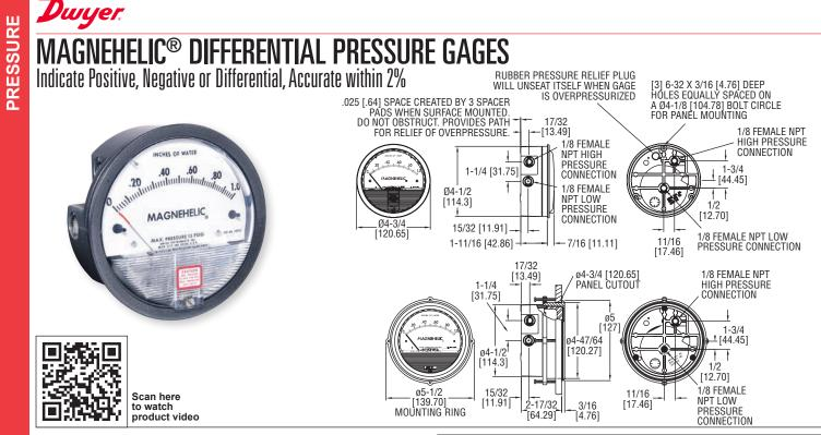
Select the SERIES 2000 Magnehelic® Gage for high accuracy--guaranteed within 2% of full scale--and for the wide choice of 81 models available to suit your needs precisely. Using Dwyer's simple, frictionless Magnehelic® gage movement, it quickly indicates low air or non-corrosive gas pressures--either positive, negative (vacuum) or differential. The design resists shock, vibration and over-pressures.
