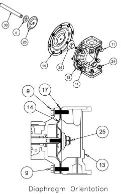
Install diaphragm and spacer as shown above.
