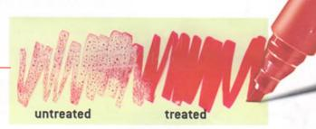
In this way the surface energy of a material can be determined to be between two values, e.g. between 36 and 38 mN/m.
