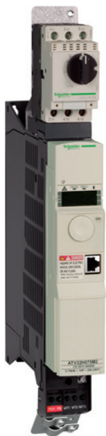
GV2/ATV32 direct mounting: GV2L08 + (VW3A9921 + GV2AF4) (3) + ATV32H075N4
