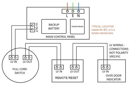
\* Wiring with 0.75/1.0mm2 2-cores alarm cable
