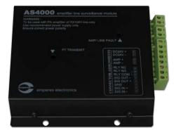
AS4000 is used to monitor the status of 70 / 100V line power amplifiers which do not have built in detection module. Every amplifier shall employ one AS4000 and the dry contact output from the unit shall then be connected to Amperes AC3801. Repeating this link shall then form an automatic amplifier fault changeover / surveillance system.
