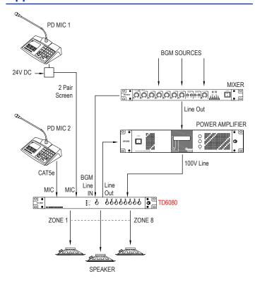
Typical configuration of TD6080 as zone decoder  $\!\!/$  selector.
