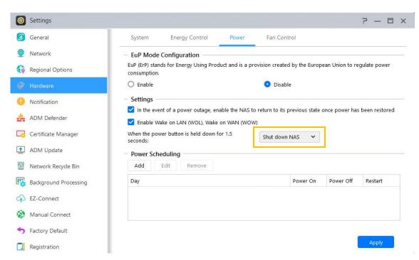
2. Hold down the power button for 1.5 seconds. You should be able to hear a "beep" from the system buzzer. Let go of the power button and the NAS will either shut down or enter sleep mode depending on your configuration.
