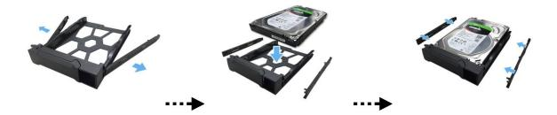
✓ To install a 2½" hard drive, please remove the two rails on both sides of the hard drive tray. Align the hard drive with the 4 holes labeled 2.5" with the SATA connector facing outward. While maintaining a grip on the hard drive and tray, turn the tray upside down and secure the drive with four included M3 screws as demonstrated below.
