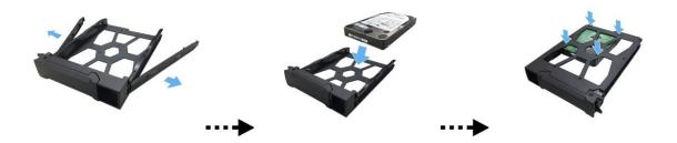
4. Slide the disk tray onto the rails of the disk bay. Using the latch, gently push the disk tray all the way into the disk bay. Secure the disk tray in place by pushing down on the latch. The latch should close easily and snap in with an audible 'click'. Please make sure that the disk tray is pushed all the way into the disk bay before attempting to secure the latch.
