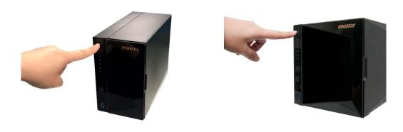
4. The NAS is ready for operation once the green system status LED indicator has stopped flashing and remains steadily lit. At this time, you should also hear a 'beep' from the system buzzer. Hardware installation is now complete. Please move on to the software installation guide to configure your system settings.
