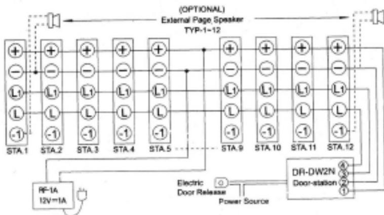
Figure-5 TP-nRC and DR-DW2N Connection Diagram
