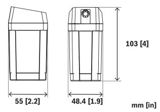
Fig. 3: Subwoofer adapter for EVOLVE-WMK with Phoenix-style connector
