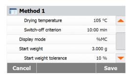
Press **Start weight tolerance** to set the tolerance of the Target weight.
