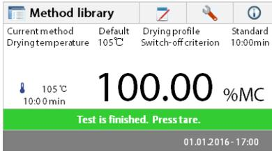
The display indicates the Method Name, Temperature/Time, actual temperature, elapsed time duration of the test, moisture and curve. The test automatically stops at the end of the measurement.
