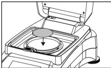
Place the empty sample pan and glass fiber pan in the pan handle. The sample pan must lie flat in the pan handle.
