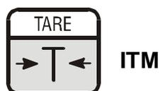
This button is used to temporarily set the scale to zero (such as canceling the weight of a carton before performing a filling operation). The display will show NET weight and the NET annunciator will be lit.
