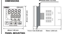
10001 10001 1-Before mounting the device in your panel, make sure that the panel cut-out is suitable.
