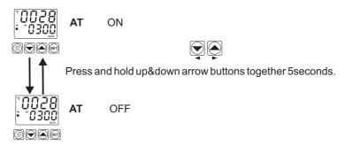
While pressed up&down arrows together 5 seconds AT led will active and AUTO TUNE starts. Motorized valve will go to minimum and maximum points for identify autotone. For a while Auto tune finish and proportional band starts.
