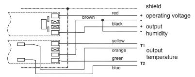
Pin assignment sensors IRC..., ITC.. Humidity active, temperature passive
