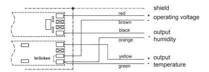
Pin assignment sensors IRK..., ITK.. Humidity active, temperature active
