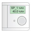
Setpoint 1 for Relay 1 adjustable with rotary selector
