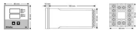
Panel cut-out =  $45 \times 45 \text{ mm}$
