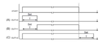
E-55 Series Timer is a single output general purpose timer which can be easily configured by the user. The start signal is generated upon applying 220 V AC to the START inputs. The output forms depending upon the "out" parameter are shown above.
