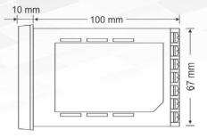
Panel cut-out =  $68 \times 68 \text{ mm}$
