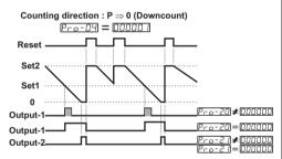
3:Manual Reset-3:Device continues to count till manual reset is applied. (Output-2 pulse time Pco-21) is not considered.)
