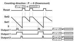
2:Manual Reset-2:Counting does not continue over SET2 value.For starting to count manual reset input must be active. Output-2 pulse time Pro-21 is not considered.
