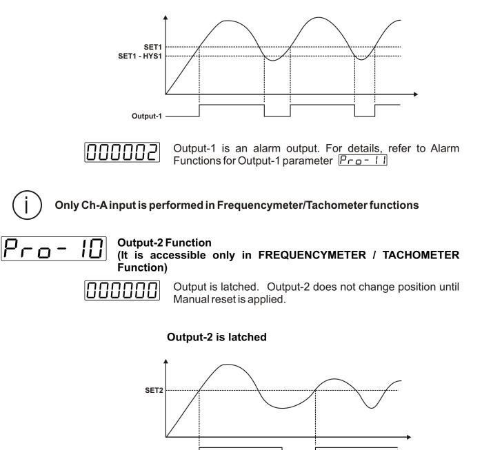
Only Ch-A input performs in Frequencymeter / Tachometer function.
