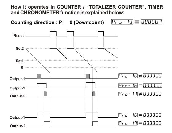
When the count value reaches to SET1 value, Output-1 becomes active. If Output-1 pulse time  $P_{ro}$  - 16 is not 0, Output-1 changes position at the end of the pulse time. If Output-1 Pulse Time  $P_{ro}$  - 16 is 000000 it changes position until Manual Reset input is active or according to Output-2.
