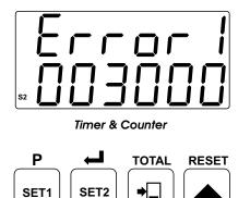
**1** - Position of the DIP Switch is wrong. (DIP Switch determines the operation function of the device and it is under the top cover)
