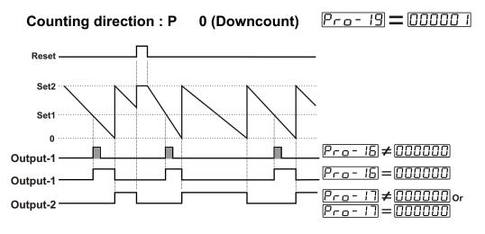
If count value is equal to or less than SET1 value, then Output-1 becomes active. If Output-1 pulse time  $P_{ro} - I_{D}$  is not 0, Output-1 changes position at th end of the pulse time. If Output-1 pulse time
