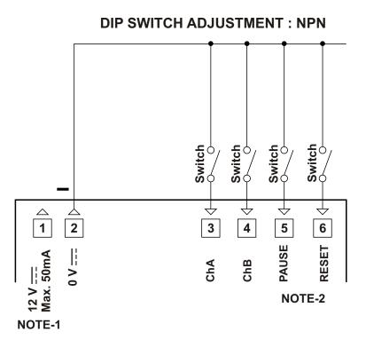
NOTE-1 : Auxiliary power supply for external transmitter 12V\_\_\_\_\_ ± 10%, 50 mA maximum short circuit protection
