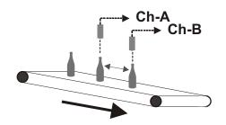
When the object passes in front of the first sensor on Ch-A input, counting is started (Minute / second).
