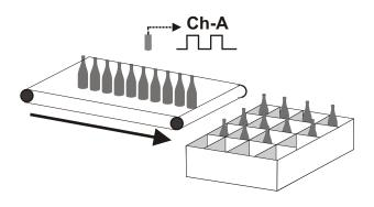
Device is used in a packing line as shown on the left. Bottles must be counted into packs of 4 bottles and dispatched in a box containing a batch of 4 packs. According to this, SET1 and SET2 are defined 4. 4 pieces of packet which contain a batch of 4 series are allowed to be formed.
