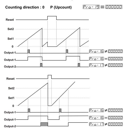
When the count value reaches to SET1, Output-1 becomes active. If Output-1 pulse time  $P_{ro}$  -  $I_{D}$  is not 0, Output-1 changes position at the end of the pulse time. If Output-1 Pulse Time  $P_{ro}$  -  $I_{D}$  is 000000, it changes position until Manual Reset input is active or according to Output-2 position.
