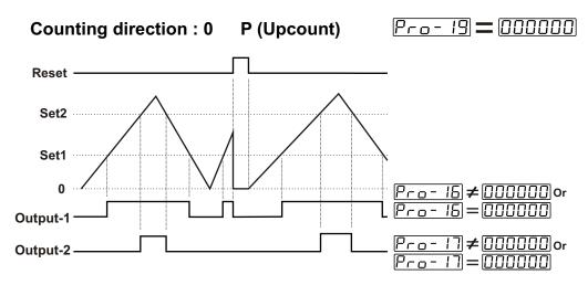
If count value is equal or greater than SET1 value, then Output-1 becomes active. Output-1 pulse time  $P_{ro} - I_{D}$  is not considered.
