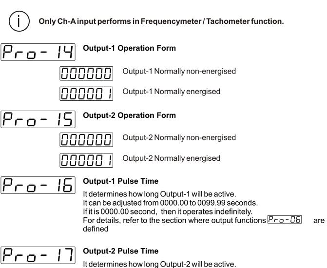
It determines now long Output-2 will be active. It can be adjusted from 0000.00 to 0099.99 seconds. If it is 0000.00 second, then it operates indefinitely. For details, refer to the section where output functions  $P_{\Box} = \Box \Box$  are defined
