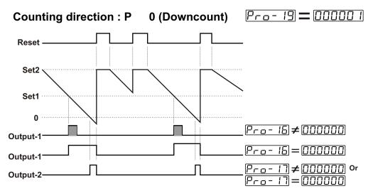
When the count value reaches to SET1 value, Output-1 becomes active. If Output-1 Pulse Time  $P_{ro}$  - 16 is 000000, Output-1 does not change condition until manual reset input is active. If Output-1 pulse time  $P_{ro}$  - 16 is not 0, Output-1 becomes inactive at the end of the pulse time. When actual value reaches to 000000, Output-2 becomes active. Counting countinues under 0000000 Output-2 pulse time  $P_{ro}$  - 17 Is not considered.
