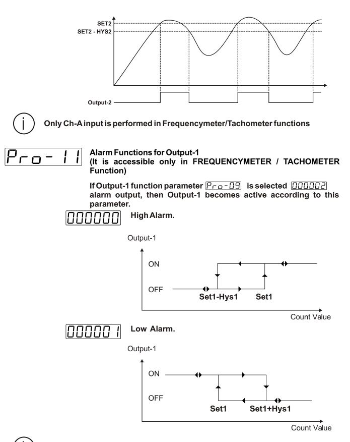
Only Ch-A input performs in Frequencymeter / Tachometer function.
