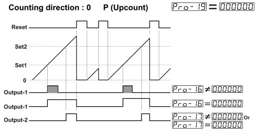
When count value reaches to SET1 value, Output-1 becomes active. If Output-1 pulse time  $P_{r_{D}} - I_{D}$  is  $\boxed{\Box \Box \Box \Box \Box \Box}$ , Output-1 does not change condition until manual reset input is active. If Output-1 pulse time  $P_{r_{D}} - I_{D}$  Is not 0, at the end of the pulse time Output-1 becomes inactive. When count value reaches to SET2 value, Output-2 becomes active. Counting continues over SET2 value. Output-2 pulse time  $P_{r_{D}} - I_{D}$  Is not considered.
