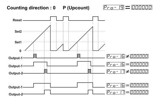
When the count value reaches to SET1 value, Output-1 becomes active. If Output-1 Pulse Time  $P_{ro} - I_{D}$  is not 0, Output-1 changes position at the end of the pulse time. If Output-1 Pulse Time  $P_{ro} - I_{D}$  is  $\boxed{000000}$  to changes position until Manual Reset input is active or according to Output-2.
