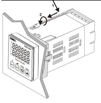
The unit is designed for panel mounting.
