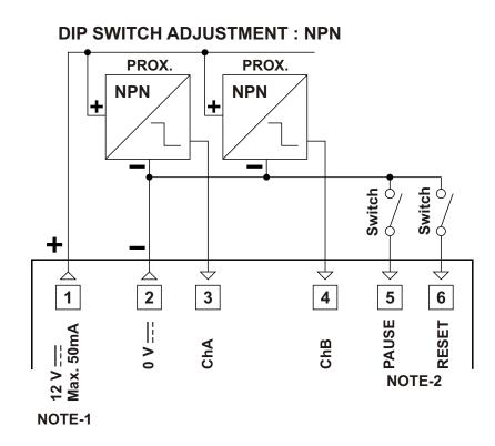
NOTE-1 : Auxiliary power supply for external transmitter  $12V_{---} \pm 10\%$ , 50 mA maximum with short circuit protection
