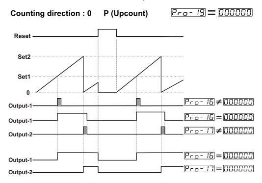
When the count value reaches to SET1 value, Output-1 becomes active. If Output-1 pulse time  $P_{ro} - I_{D}$  is not 0, Output-1 changes position at the end of the pulse time. If Output-1 Pulse Time  $P_{ro} - I_{D}$  is  $\Box \Box \Box \Box \Box \Box$ , it changes position until Manual Reset input is active or according to Output-2 position.
