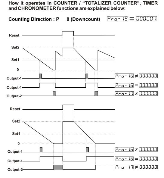
When the count value reaches to SET1, Output-1 becomes active. If Output-1 pulse time  $P_{ro}$  -  $I_{B}$  is not 0, Output-1 changes position at the end of the pulse time. If Output-1 Pulse Time  $P_{ro}$  -  $I_{B}$  is 000000, it changes position until Manual Reset input is active or according to Output-2 position.
