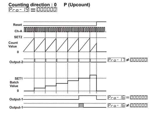
When count value reaches to SET2 value, count value is reset and Output-2 becomes active. If Output-2 pulse time  $P_{-p-17}$  is  $\boxed{DDDDD}$  Then Output-2 does not change position until manual reset input is active. If Output-2 pulse time  $\boxed{P_{-p-17}}$  is not 0, Output-2 becomes inactive at the end of the pulse time.
