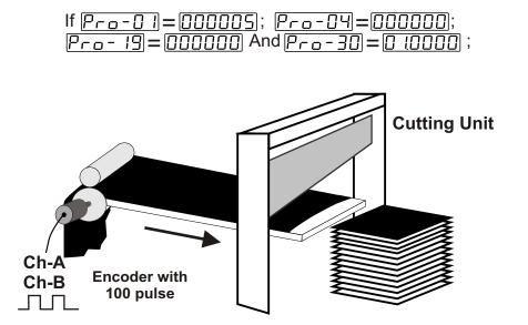
Coefficient parameter is adjusted to be able to observe the cloth length in actual value screen. If we want to be cut the cloth in same lenght at 5 m and stopped the system when 40 pieces of 5 m cloths are formed, SET1 must be 40 and SET must be 5.
