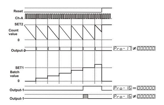
When count value reaches to  $\boxed{\Box \Box \Box \Box \Box \Box \Box}$ , count value becomes equal to SET2 and Output-2 becomes active. If Output-2 Pulse Time  $\boxed{P_{ror} - 1}$  is  $\boxed{\Box \Box \Box \Box \Box}$ , then Output-2 does not change position until manual reset input is active. If Output-2 pulse time  $\boxed{P_{ror} - 1}$  is not 0, then Output-2 becomes inactive at the end of the pulse time.
