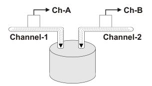
If the tank is filled with liguid 20 liters from Channel-1 and 40 liters from Channel-2, 60 liters is observed in actual value screen.
