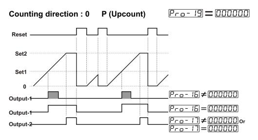
When the count value reaches to SET1 value, Output-1 becomes active. If Output-1 pulse time  $P_{ro} - I_{5}$  is  $D_{D} D_{D} D_{0}$ , Output-1 does not change position until manual reset input is active. If Output-1 pulse time  $P_{ro} - I_{5}$  is not 0, Output-1 becomes inactive at the end of the pulse time.
