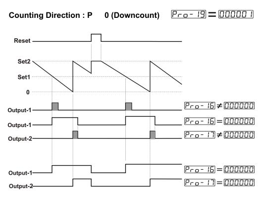
When the count value reaches to SET1 value, Output-1 becomes active. If Output-1 pulse time  $P_{ro} - I_{D}$  is not 0, Output-1 changes position at the end of the pulse time. If Output-1 Pulse Time  $P_{ro} - I_{D}$  is 000000 it changes position until Manual Reset input is active or according to Output-2 position.
