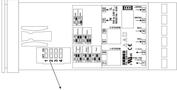
DIP Switch is under cover and cover is on top side of the device
