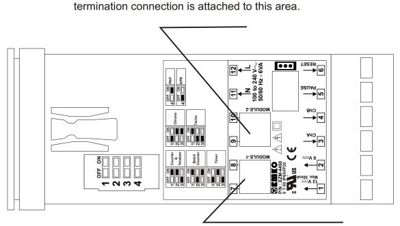
Label which is plugged in Module-1 socket, describes module termination connection is attached to this area.
