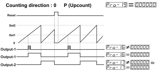
If count value is equal to or greater than SET1 value, then Output-1 becomes active. If Output-1 pulse time Pro-IB is not 0, Output-1 changes position at the end of the pulse time. If Output-1 pulse time Pro-IB Is DDDDD, then Output-1 becomes inactive when count value reaches to SET2 value.
