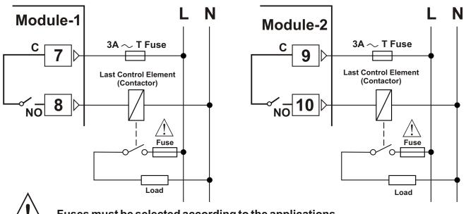
Fuses must be selected according to the applications.
