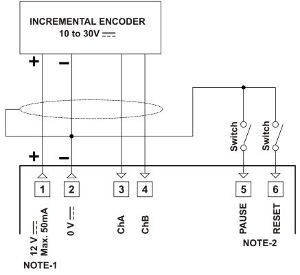
NOTE-1 : Auxiliary power supply for external transmitter  $12V_{---} \pm 10\%$ , 50 mA maximum short circuit protection
