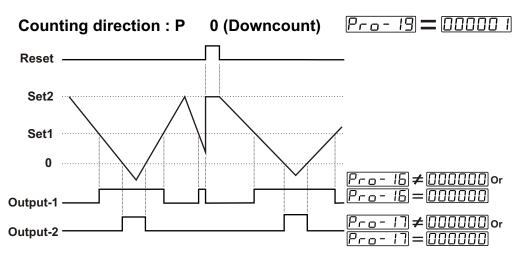
If count value is equal or less than SET1 value, then Output-1 becomes active. If it is greater than SET1 value, Output-1 becomes inactive. Output-1 pulse time  $P_{ro} - I_{D}$  is not considered.
