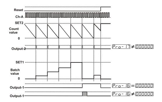
When count value reaches to  $\boxed{\Box \Box \Box \Box \Box \Box}$  value, count value becomes equal to SET2 value and Output-2 becomes active. If Output-2 pulse time  $\boxed{P_{r \Box} - I}$  is  $\boxed{\Box \Box \Box \Box \Box}$ , then Output-2 does not change position until manual reset input is active. If Output-2 pulse time  $\boxed{P_{r \Box} - I}$  is not 0, Output-2 becomes inactive at the end of the pulse time.
