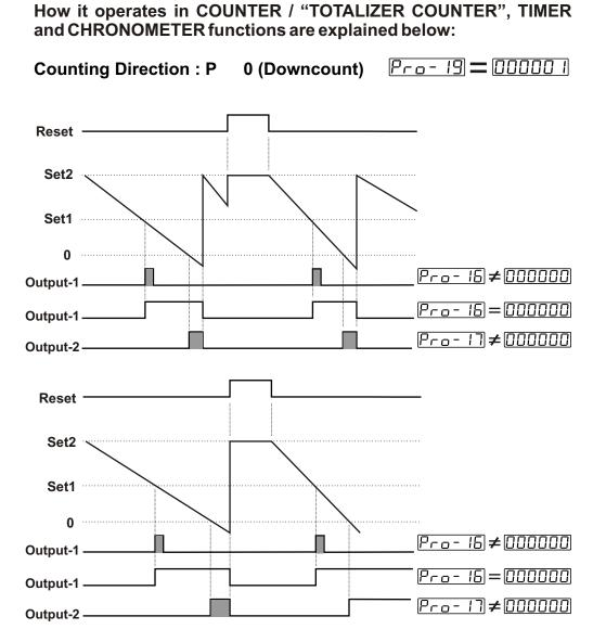
When the count value reaches to SET1, Output-1 becomes active. If Output-1 pulse time  $P_{\_\_\_\_\_\_16}$  is not 0, Output-1 changes position at the end of the pulse time. If Output-1 Pulse Time  $P_{\_\_\_\_\_\_16}$  is  $\boxed{000000}$ , it changes position until Manual Reset input is active or according to Output-2 position.
