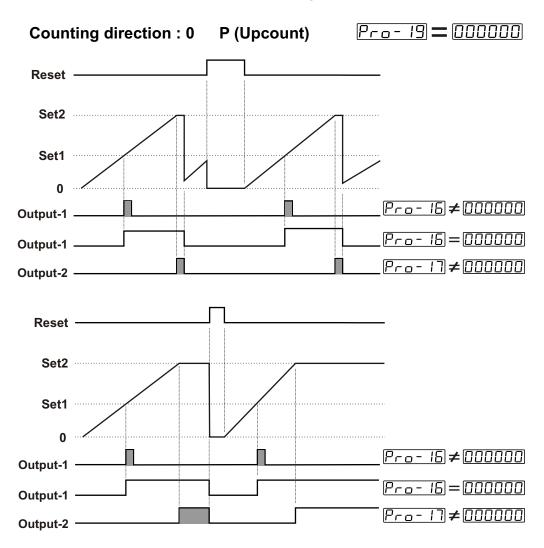
When the count value reaches to SET1, Output-1 becomes active. If Output-1 pulse time  $P_{ro}$  -  $I_{6}$  is not 0, Output-1 changes position at the end of the pulse time. If Output-1 Pulse Time  $P_{ro}$  -  $I_{6}$  is DDDDDD, it changes position until Manual Reset input is active or according to Output-2 position.
