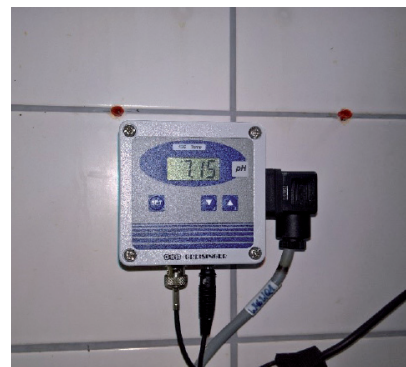
The display of the transducer can be temporarily switched to temperature display
