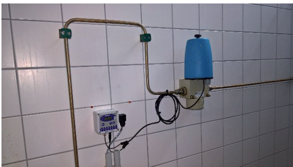
pH measurement upstream and downstream from the water treatment plant. The pH electrodes were integrated into existing sampling points.
