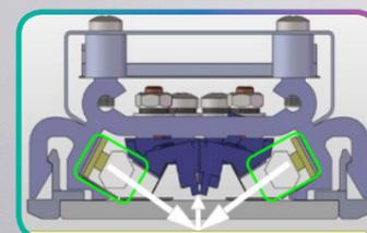
Bi-directional illumination from dual LED arranged on the right and left of the sensor reduces shadowing at creases or folds. High quality scanned image can be obtained.
