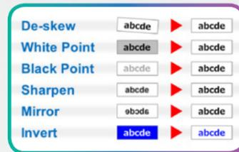
Abundant image enhancement features are incorporated such as de-skew, white point, color reversal of diazo print and restoration of deteriorated original images, which is useful for archiving old drawings.
