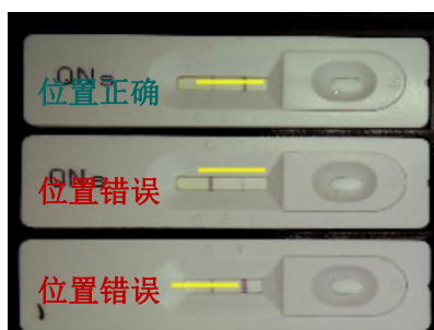
Picture 7-4 Correct position of yellow line
