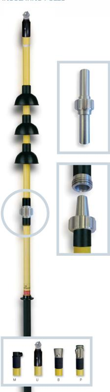
Connectable pole with two or three sections made with polyester and fibreglass tube Ø 40 mm with hand protector, grip, tip, 3 deflecting hoods and M (Metric-10), U (Universal), B (Bayonet) or P (Hexagonal + Metric-10) head.
