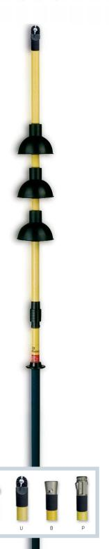
Connectable pole with two sections made of polyester and fibreglass tube  $\emptyset$  32 mm with humidity-proof seals on each end, hand protector, grip, tip, 3 deflecting hoods and M (Metric-10), U (Universal), B (Bayonet) or P (Hexagonal + Metric-10) head.
