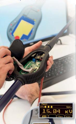
Bipolar voltage detector with digital display OLED to be used in MV netwoorks.
