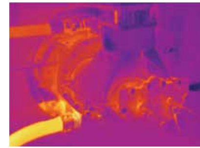
Limited temperature increase of only 25°C inside compressor element
