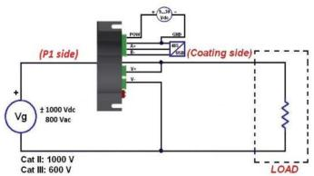
**CAUTION:** Magnetic fields of high intensity can vary the values measured by the transformer. Avoid installation near permanent magnets, electromagnets or iron masses that induce strong changes in the magnetic field. If any irregularity recommend reorient or move the transformer in the area most appropriate.
